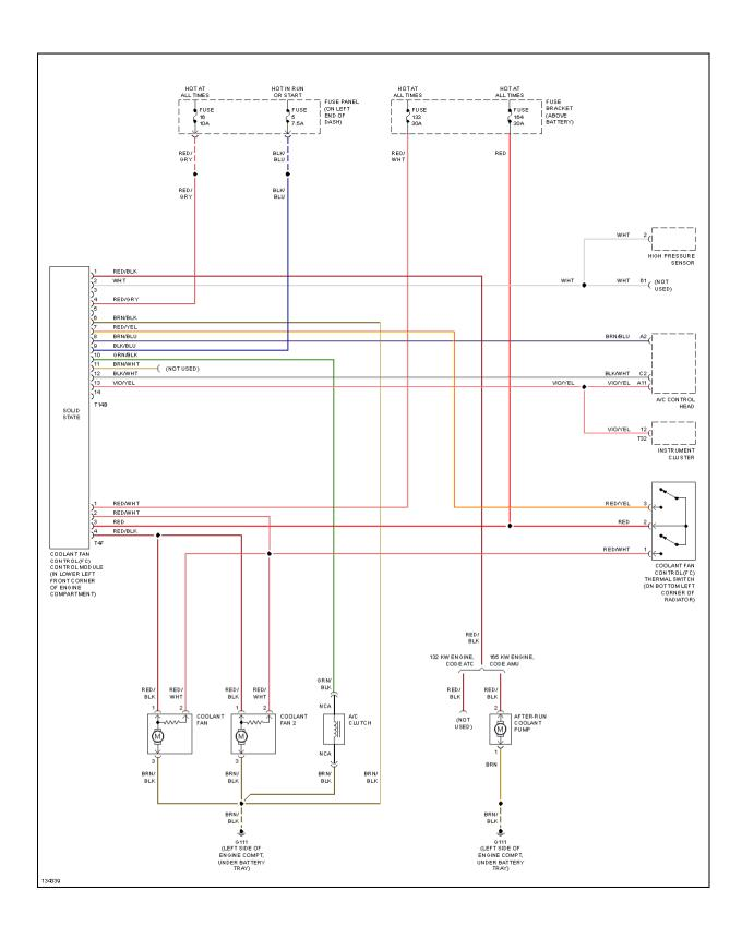
Fig. 9: Cooling Fan Circuit
