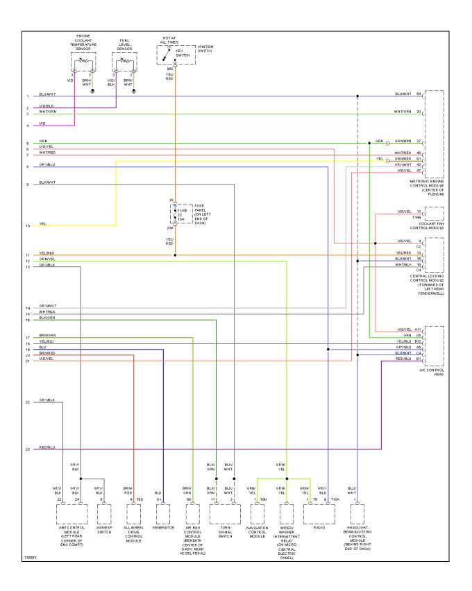
Fig. 30: Instrument Cluster Circuit (2 of 2)
