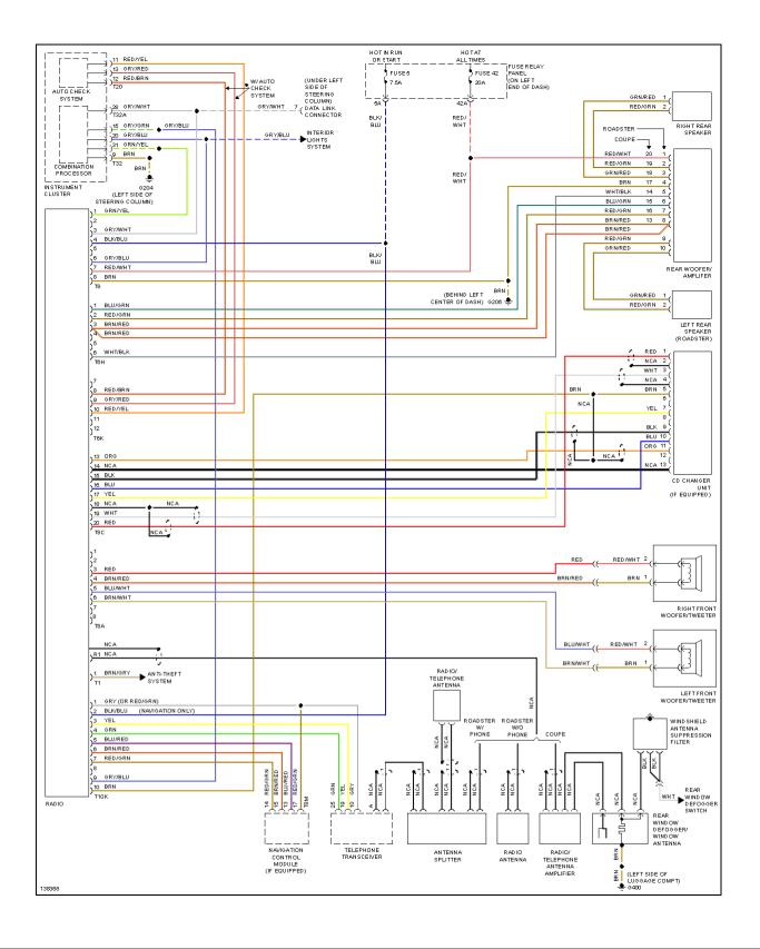
Fig. 46: Radio Circuit, W/O Bose System
