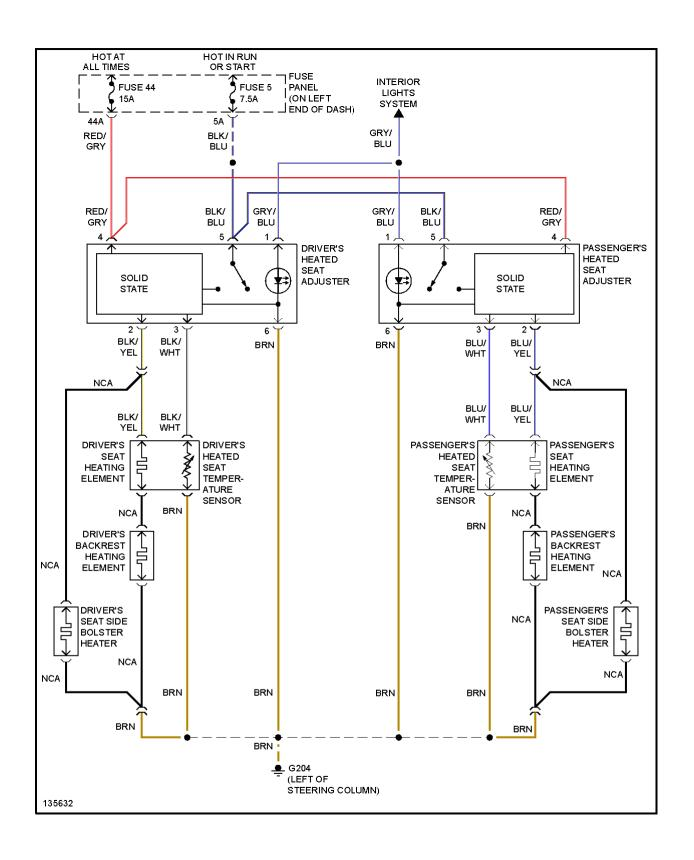
Fig. 42: Heated Seats Circuit
