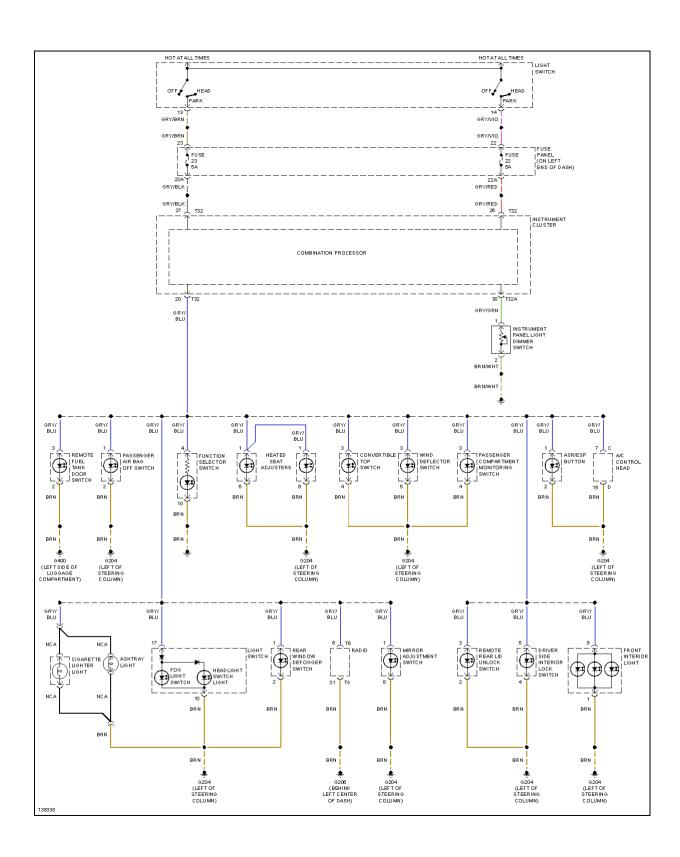
Fig. 32: Instrument Illumination Circuit
