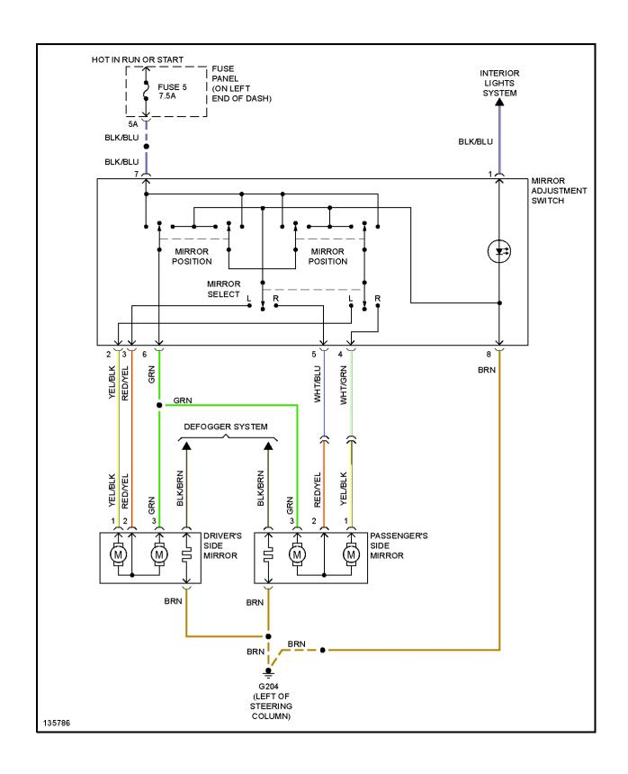
Fig. 41: Power Mirrors Circuit
