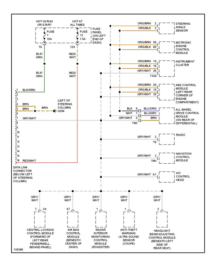
Fig. 8: Computer Data Lines Circuit
