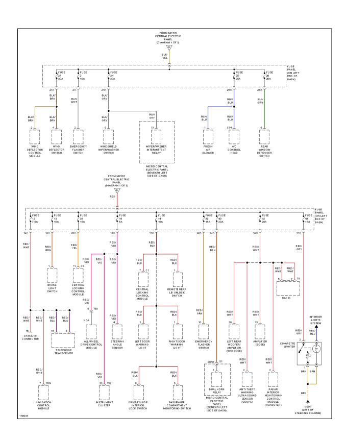
Fig. 36: Power Distribution Circuit (3 of 3)
