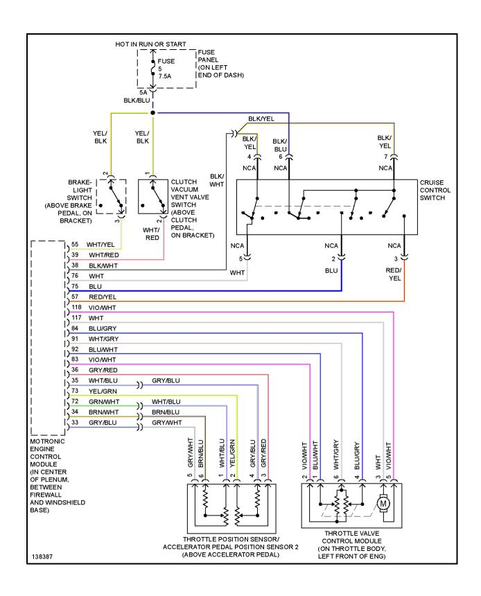
Fig. 10: Cruise Control Circuit
