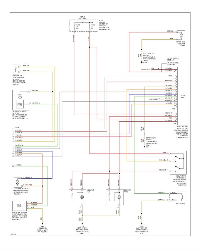
Fig. 2: Automatic A/C Circuit (2 of 2)
