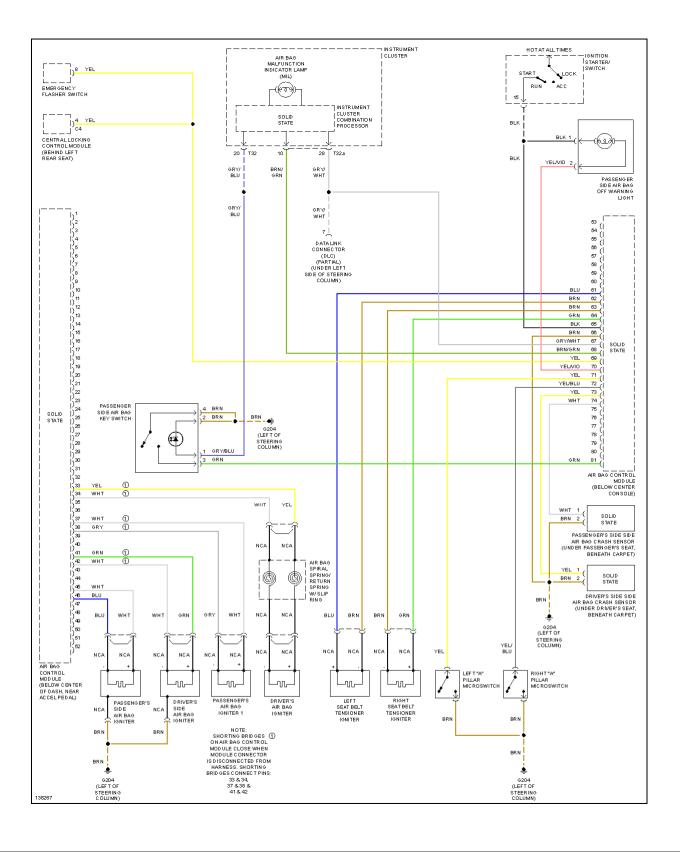
Fig. 49: Supplemental Restraints Circuit
