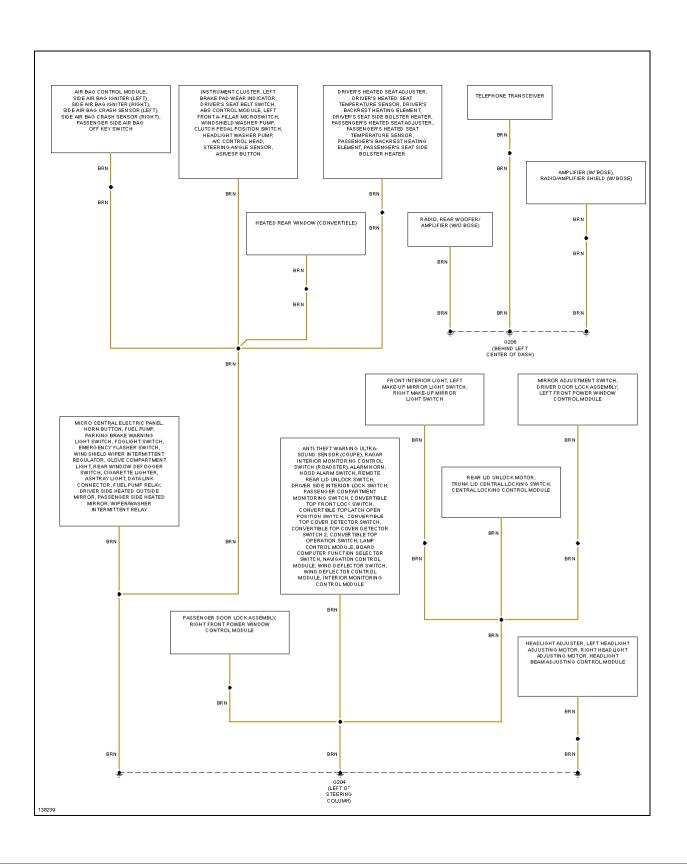
Fig. 22: Ground Distribution Circuit (2 of 2)
