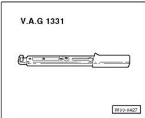
**Fig. 209: Torque Wrench V.A.G 1331**
