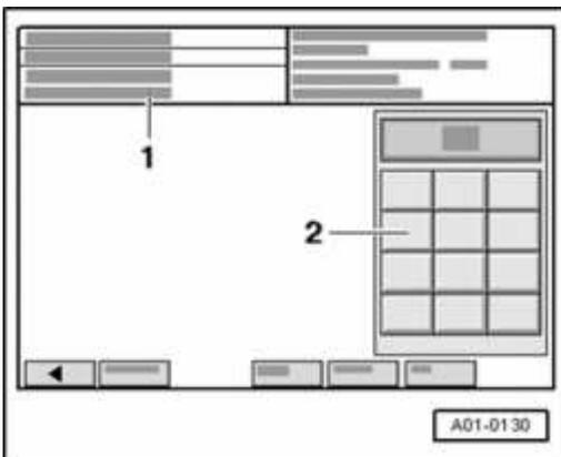
**Fig. 21: Diagnostic System VAS 5051: Display - Display Group And Key Pad**
