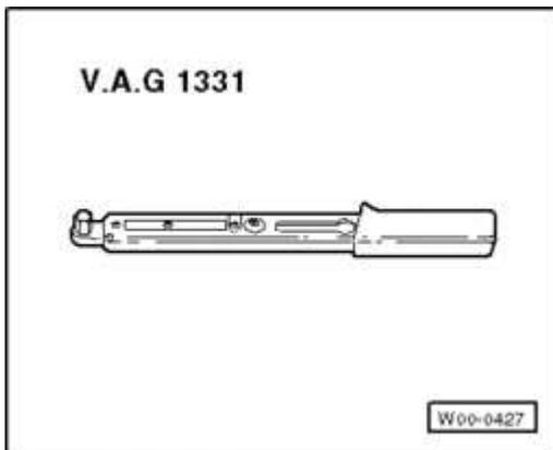
**Fig. 101: Torque Wrench V.A.G 1331**
