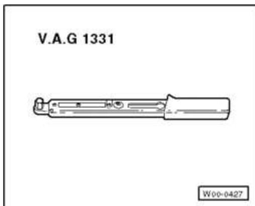
**Fig. 89: Torque Wrench V.A.G 1331**
