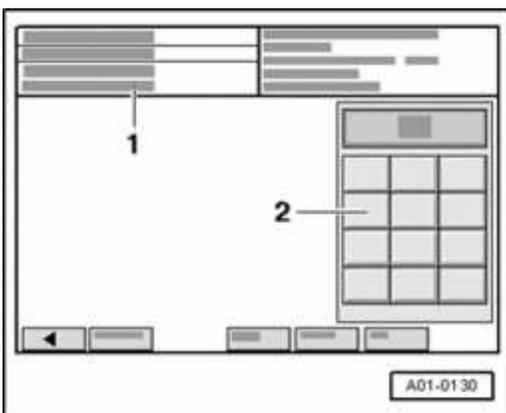
**Fig. 34: Diagnostic System VAS 5051: Display - Display Group And Key Pad**
