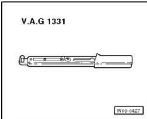
**Fig. 117: Torque Wrench V.A.G 1331**
